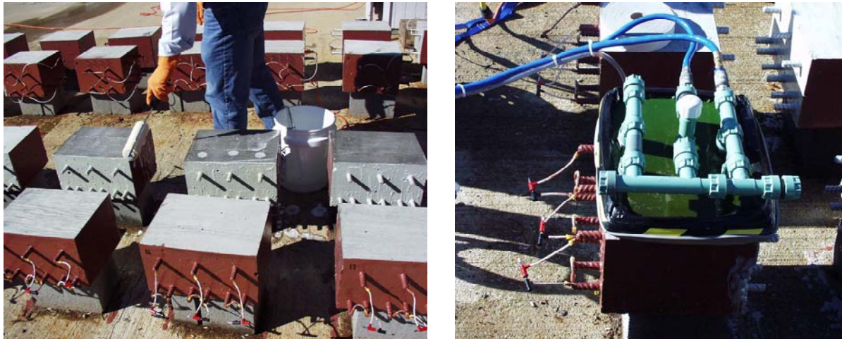
Figure 3. (a) Inhibitor applied using roller. (b) Inhibitor applied using vacuum/pressure injection.
