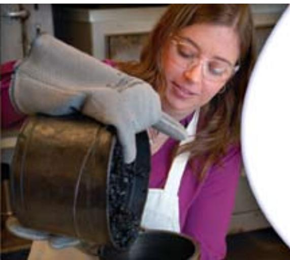
***Left:** Research Scientist Stacey Diefenderfer places a sample of warm-mix asphalt into a gyratory mold in the VTRC laboratory.*
