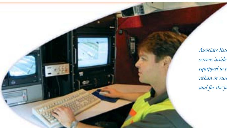
*Associate Research Scientist Lance Dougald monitors video screens inside the VTRC Smart Travel Van. The van is equipped to collect on-site, real-time traffic data from any urban or rural area in the state for Research Council projects and for the joint U.Va.-VTRC Smart Travel Lab.*
